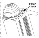
head assembly, simply unscrew the head lock  $\frac{1}{4}$  turn and rotate it counter-clockwise.
