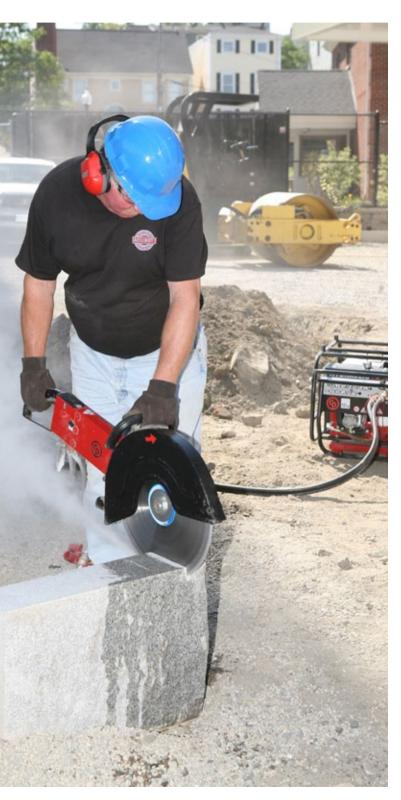
They may be light and compact, but don't be fooled. A CP hydraulic cut-off saw with the right blade will cut through concrete, asphalt and steel. With our 16-inch saw at full throttle, you have the raw power of a petrol powered engine in your hand.
