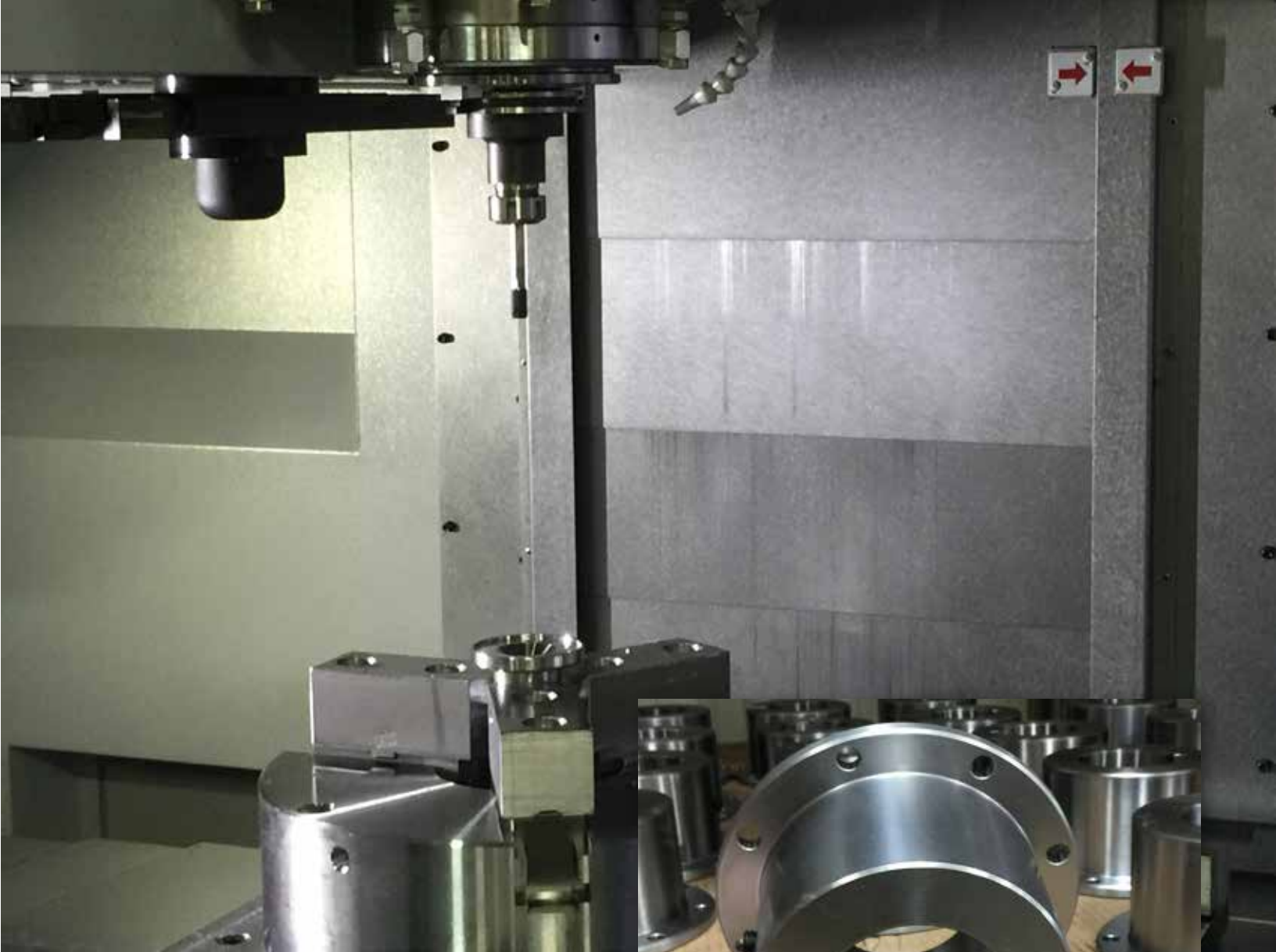
Above: The EXOPRO® OIL-S-XPF form tap was put into Ameridrives' new DMG Mori NVX 5100 for a tool life test in 8620 alloy steel.
