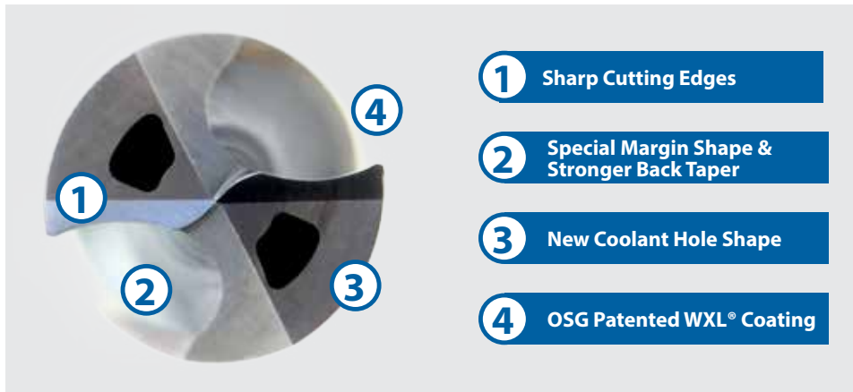
Figure 1. Features of OSG's EXOCARB® WDO-SUS Drill
