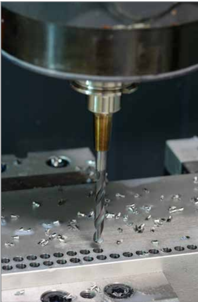
Lower cutting force and less friction for reduced cutting temperature and a new chamfer design for lower feed rates and optimal chip formation are proven results achieved by OSG with the EXOCARB® WDO-SUS coolant-through carbide drill series.
