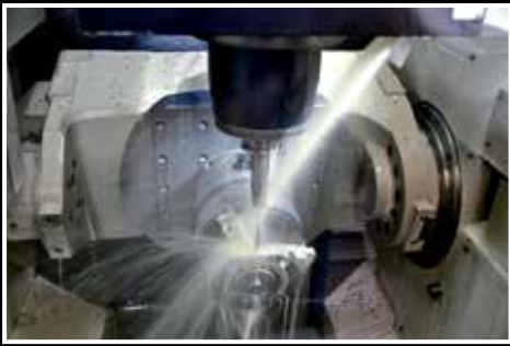
The EXOCARB® WDO-10D in action drilling at a hole depth of 58 mm in super duplex stainless steel with a 410 HB hardness.
