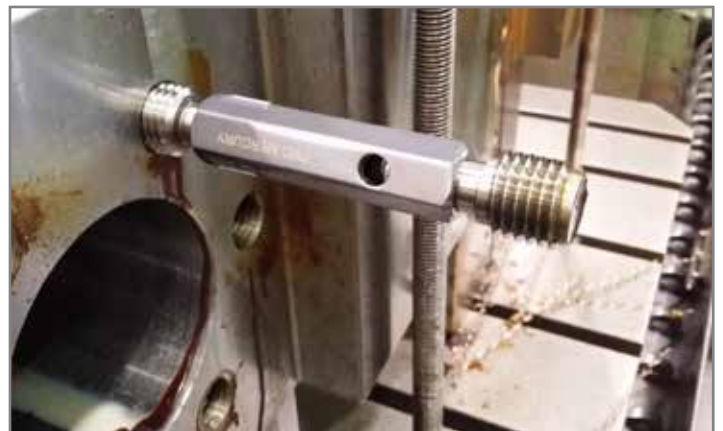
FMC's very own 1" 8UNC GO plug gauge was used to confirm the accuracy and finish of the thread surface. The thread tapped by the EXOTAP® A-TAP® Spiral Flute Tap appears in good quality.
