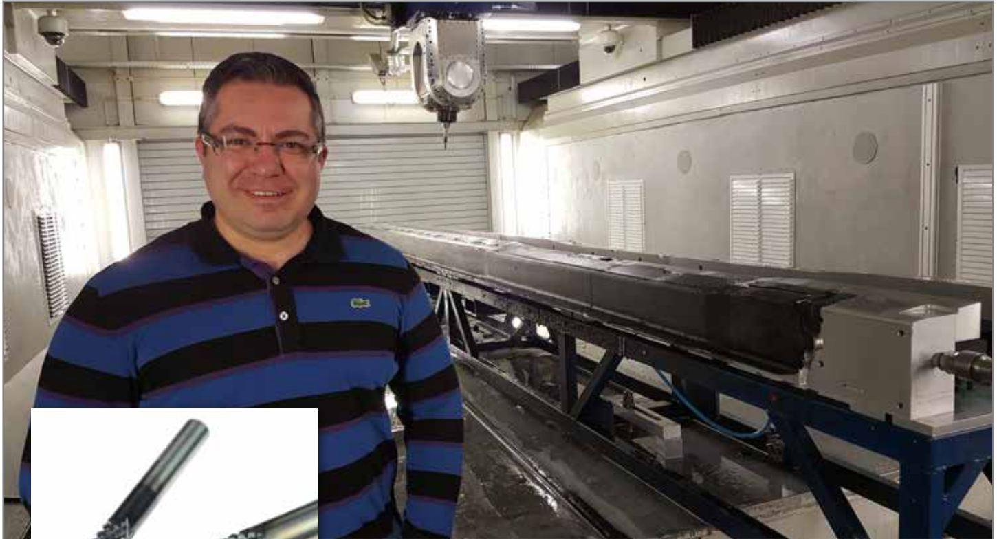
Above: The Z spars are produced in a sophisticated five-axis FOG precision milling machine. TAI's NC Engineering Leader Mr. Onur Bahtiyar oversees the production of the composite wing spars.
