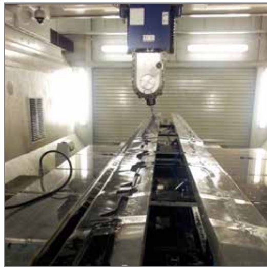
The Z spars are produced in a sophisticated five-axis FOG precision milling machine.
