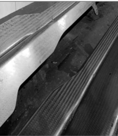
Z-shape spars that TAI has been manufacturing since 2012.
