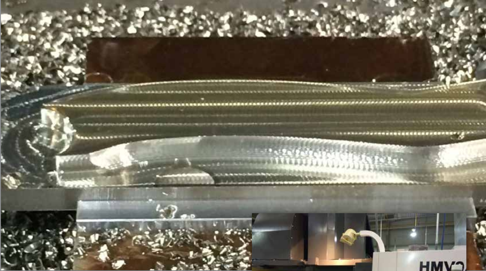
Turbine component plate in Rene 41 (40 HRC) with a dimension of 70mm x 203mm x 25.4mm.
