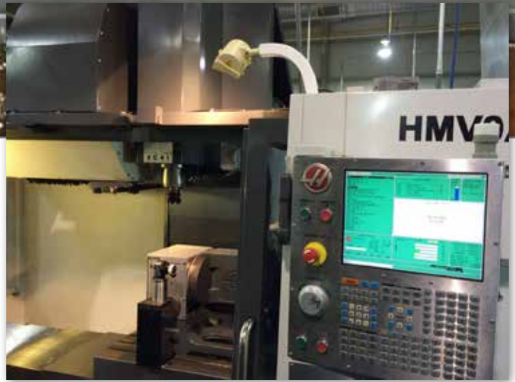
Face milling of the Rene 41 plate in Paradigm Precision's HAAS horizontal machining center using blasomill oil as coolant.
