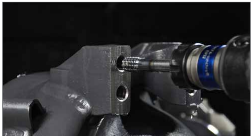
The EXOPRO® XPF is OSG's high performance form tap that produces no chips and is optimized for machining materials up to 35 HRC.
