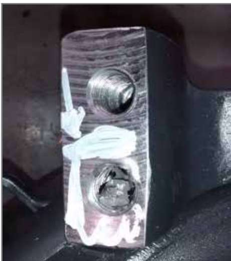
Tap breakage was a headache for Scania before switching to the EXOPRO® XPF forming tap.
