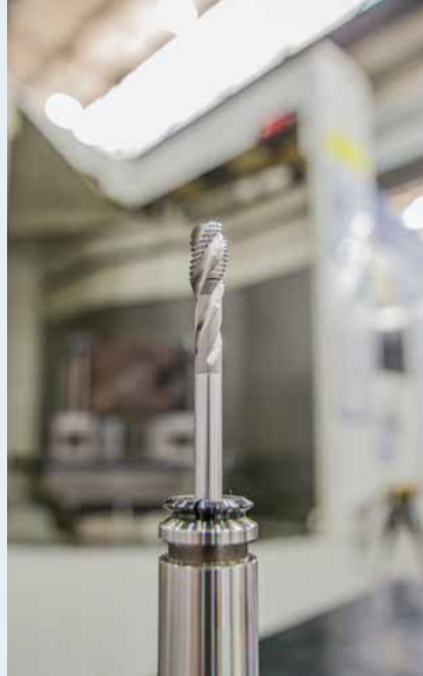
An OSG M12 x 1.75 spiral flute tap in a spindle at the production floor of B. GROB do Brasil. OSG services for GROB in all machining segments that they operate, including automotive, aerospace, mold and die, etc.
