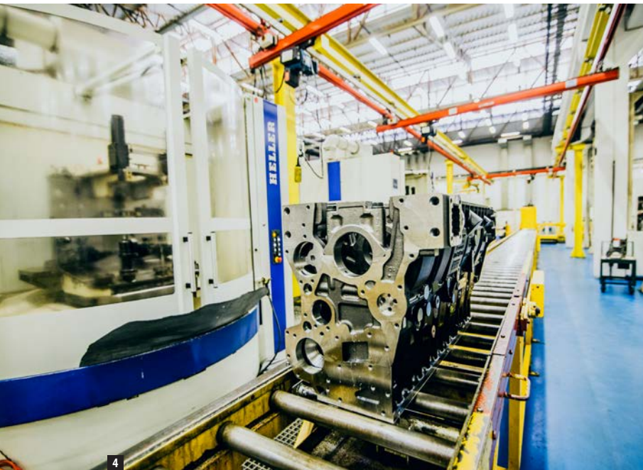
4. MWM has been producing the Acteon engine block since 2011 and manufactures approximately 3,800 blocks annually.
