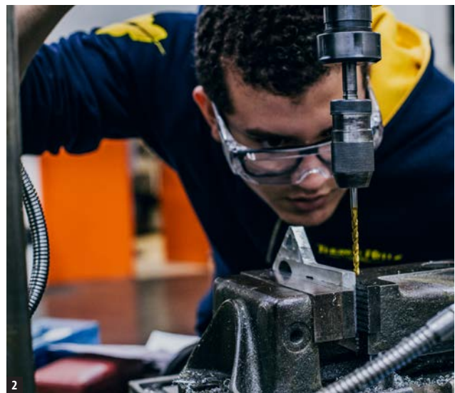
1. Julia Morone, mechanical engineering major from ThundeRatz uses an OSG hand tap to thread a robot part.
