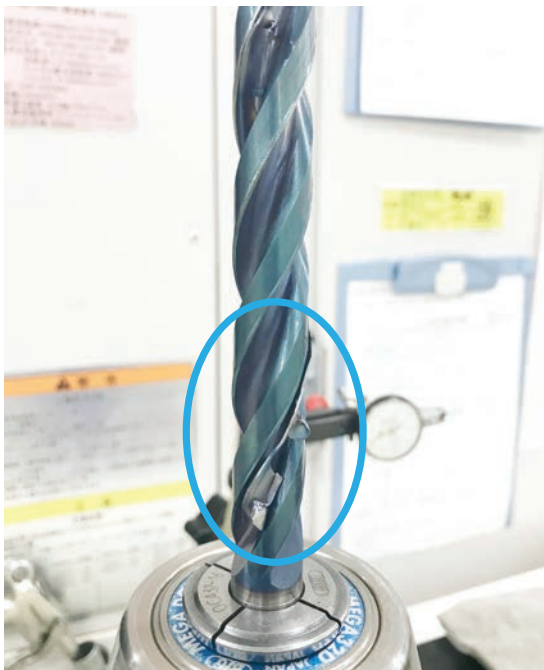
Figure 3. Condition of the conventional 3-flute drill after processing SCM440.
