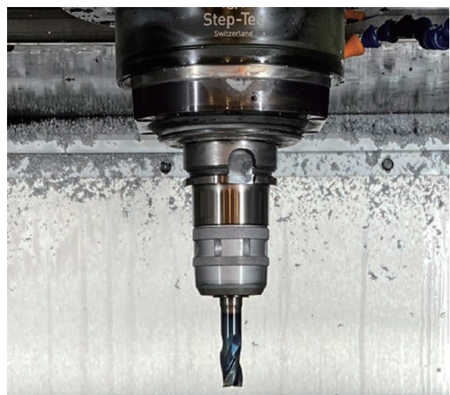
A dia. 16 R1 AERO-ETS 3-flute carbide end mill is being used at a cutting speed of 16,000 min -1 and a feed of 6,000 mm/min at a depth of cut of ap 4. OSG's AERO-ETS is one of the preferred tools for milling aluminum at Prodtek.
