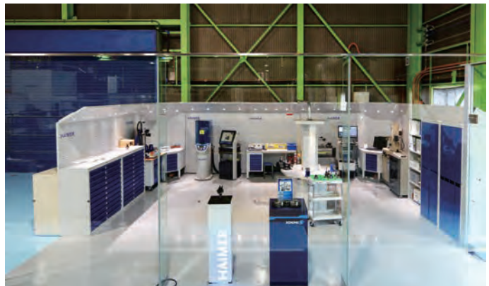
MHI installed the HAIMER Tool Management system at its Eba Factory – a working area specifically designed for tool storage, assembly, presetting and administration. Preset areas have an image of being dark and are typically situated at the corner of a factory. To eliminate this common perception, MHI purposely installed the Tool Management system as a bright, clean and open area at the factory entrance to symbolize the company's attitude toward tool management and commitment to quality.
