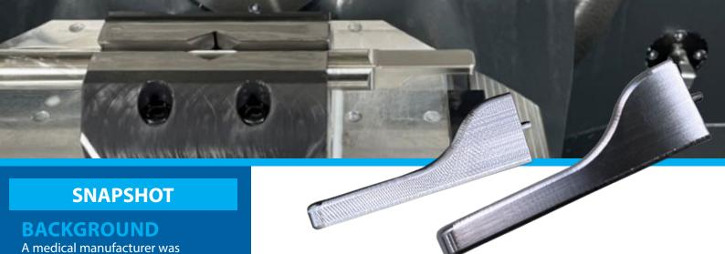
A medical manufacturer was experiencing chatter/vibration and surface finish issues while machining a part with long overhang.
