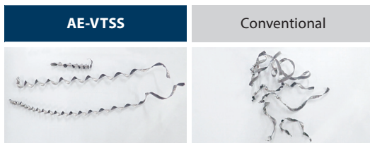
Chip shape from plunging
