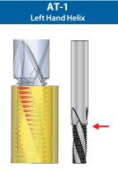
Starts cutting from the shank side Result: Reduced deflection Note: Climb milling recommended
