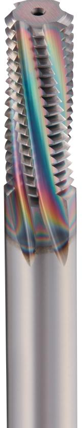
OSG's newest thread mill, the A Brand AT-1, is designed with a left-hand helix and starts cutting from the shank side, reducing deflection, preventing bending, thus allowing for 1-pass cutting and reducing overall cutting time. Along with OSG's patented EgiAs coating, it also has unequal spacing/variable lead flute which reduces vibration for better thread quality.
