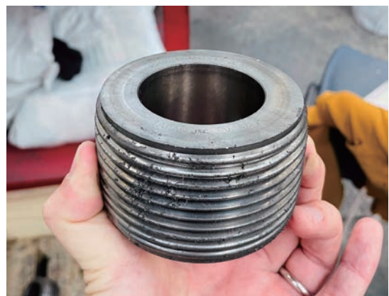
An OSG M42 x 4.5 cylindrical die. Cylindrical dies are ideal for a wide range of precision threaded parts. Thread rolling cylindrical dies are used in set of two or set of three. OSG offers customization in accordance with any desired specification.
