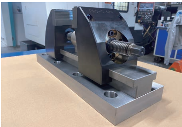
A PRO-CLAMP 5-Axis vice made by Polund, which has a long clamping distance and is ideal for all kinds of clamping associated with 5-Axis machining.
