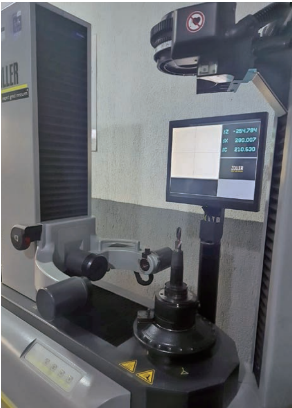
OSG's custom 2-flute carbide step drill is being preset on a Zoller tool presetter.
