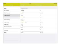
Throw off delays can be applied after the i-digits™ device is fully fabricated. The throw off delays are applied to each digit individually and are used to fine tune alignment of the digits. The delay is in the initial movement of the digits and is only applied when the digit closes from the fully open position.
