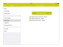
A health check of the i-limb® or i-digits™ can be completed to check the function of the device. Each digit will be moved individually. A message will be displayed on screen if there are any faults noted with the i-limb® or i-digits™ device.
