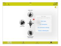
The grips programmed on the device can be returned to the default grips by choosing the hand icon to open the menu and tapping the 'reset to default grips'.
