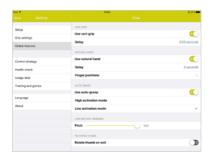
**Use pulsing:** Pulsing is the increase grip force applied by all digits at the same time. This feature can be turned on/ off. The delay is the period of time which the close signal must be sustained by the user before the pulsing feature activates.
