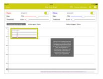
Within the training, calibration can be conducted. This allows automated set up of the timings required for the individual user. Upon selecting 'calibrate' instructions will appear on screen asking the user to generate the muscle trigger four times.
