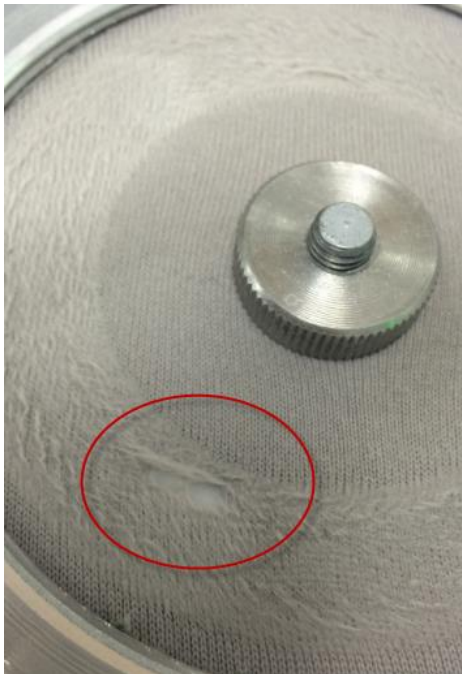
Abrasion testing: 15.000 Cycles. Hole in current suplex TT textile (Dermo Cushion)
