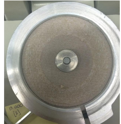
Anterior side of new textile intact after 15.000 cycles.
