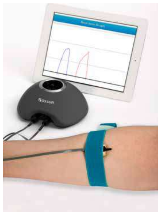
Virtu-Limb™ to measure myoelectric signals
