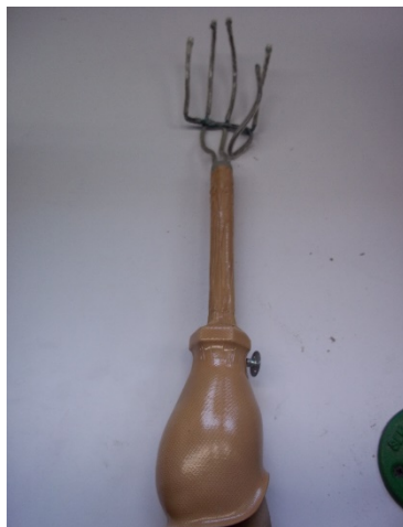
Bad socket construction- laminated pylon- should be METAL
