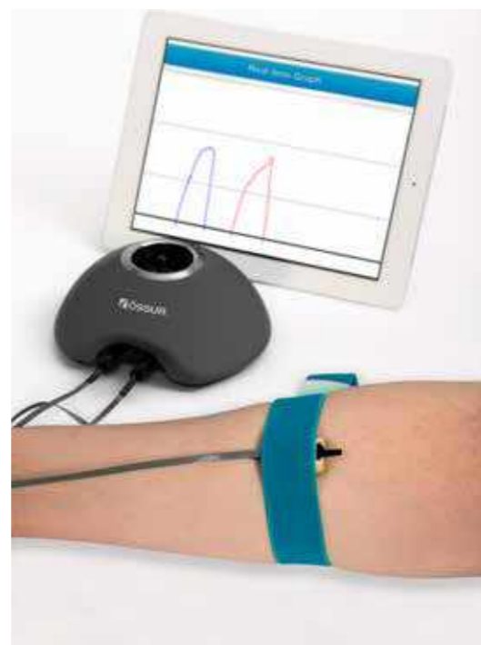
Virtu-Limb™ to measure myoelectric signals
