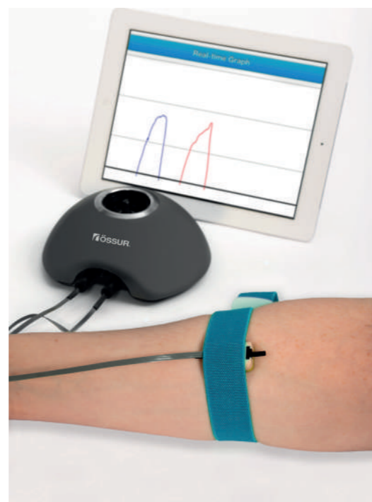
Virtu-Limb™ to measure myoelectric signals
