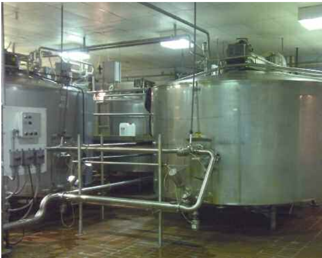
THE CHEESE VAT IS NORMALLY MADE OF STEEL AND HAS JACKETS SET TO SPECIFIC TEMPERATURES.
