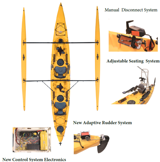
Figure 2: The components of the Tetra-Sail V1 design
