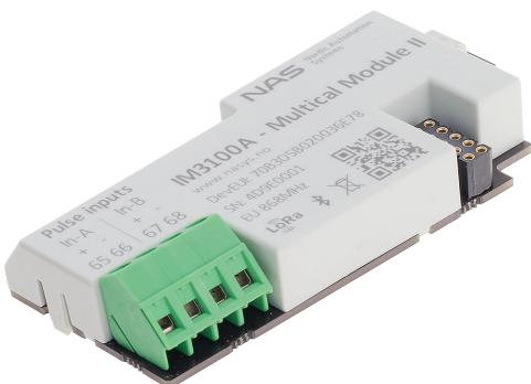
LoRaWAN™ Multical® Module II enables the acquisition of consumption data from Kamstrup Multical® series meters and transmit it wirelessly to the available LoRaWAN™ network.
