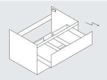
Hook vanity onto wall brackets. Mount support bracket onto wall directly under vanity base.
