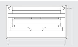
2. Drill mounting holes in wall and fasten wall brackets with screws.
