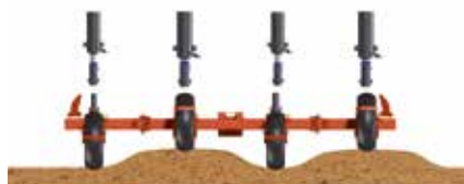
Intelligente and individual adaptation of the wheels due to the two-piece hydraulic cylinder.
