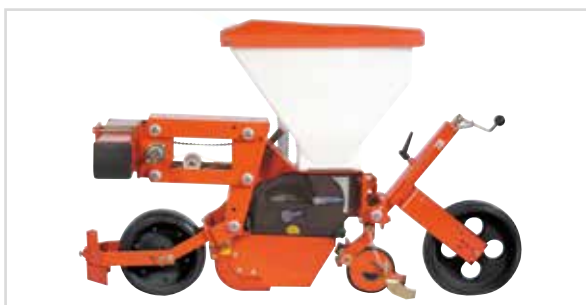
Tandem for light and marshy soil. The depth of the row is guided by the front and rear wheel.
