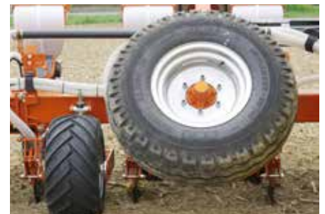
During seeding the road transport wheels are lifted up.
