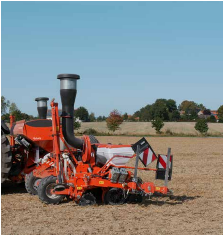
High manoeuvrability in transport due to the 90° turning cross-shaft linkage.
