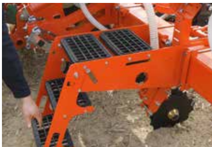
Easy access to the fertiliser hopper due to the loading step and platform.
