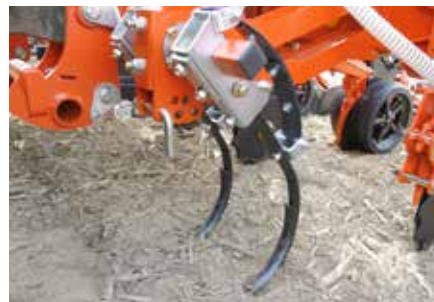
Leafspring loaded track eradicators loose compaction created by following the tracks of the tractor wheels.
