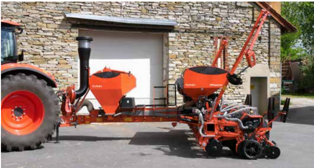
PP1601TF with SX rows and central seed hopper of 870l.
