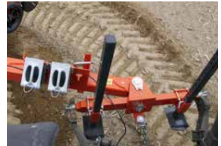
High manoeuvrability in transport due to the 90° turning cross-shaft linkage.
