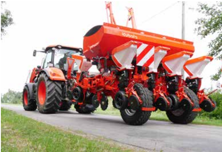
PP1601TF - Very compact in transport position. Designed for a transport speed of up to 40km/h with EU Type approval.
