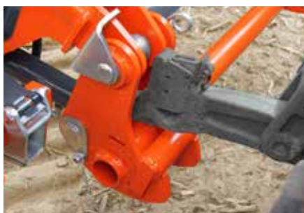
The hydraulic frame ballasting kit ensures good penetration of the sowing rows and an even sowing depth.
