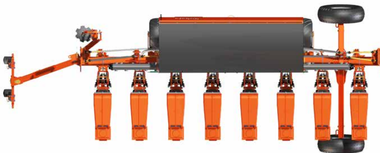
Top view in transport position. Transport width < 3m for safe road transport.
