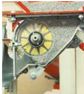
Setting for fine seeds, with rotary brush
