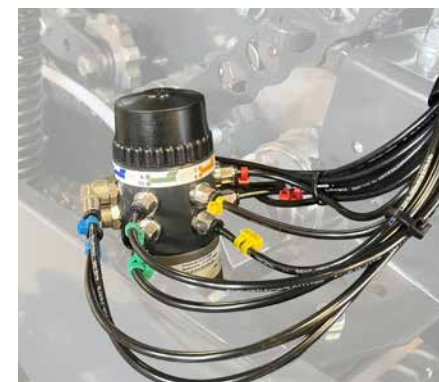
Automatic chain lubrication with individually adjustable outlets.
