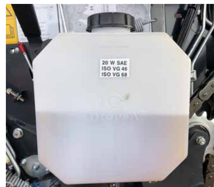
Large capacity chain lube tank.
