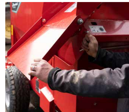
Adjustable slide for guiding material away from the wheel of the bale chopper.
