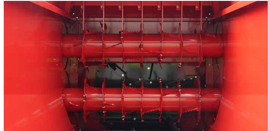
Two-drum solution designed to handle large volumes of material.
