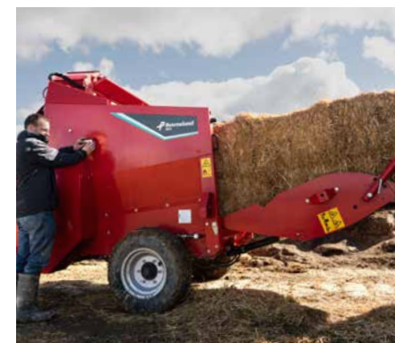
Operating both tailgate as well as floor chain in a safe distance from the moving parts by using the remote control placed on the side of the 860 series.
