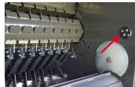
Moisture sensor located inside the bale chamber.
