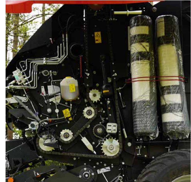
The vertical net roll storage gives an easy access to the transmission of the baler.
