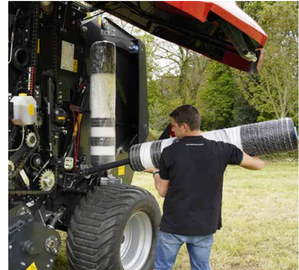
The smart net roll storage allows a comfortable horizontal loading.
