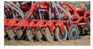
Thanks to the very slim design of the **CD coulter**, there is only a small amount of soil being moved. Therefore you need less pressure to achieve the right seeding depth. Thus, more of the available coulter pressure can be led to the press wheels. The result is a very even seed application.
