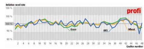
Seed rate is pretty consistent across the width of the drill, showing maximum errors of 12% (OSR), 7% (wheat) and 7% (grass). Graph: ST.
