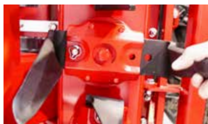
The Quick-Fit tines makes is easy to exchange without any tools.
