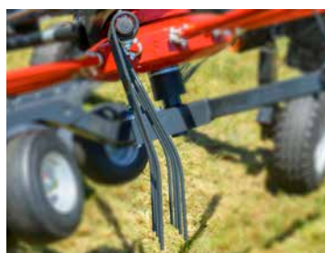
DuoTines providing perfect raking quality with raking in two rows.
