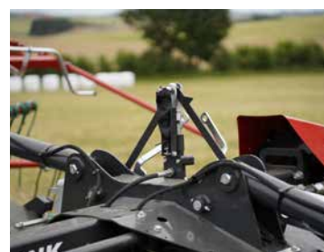
Optional hydraulic locking devices allow to unfold without opening the cabin or pulling a rope.
