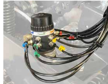
Automatic chain lubrication with individually adjustable outlets.
