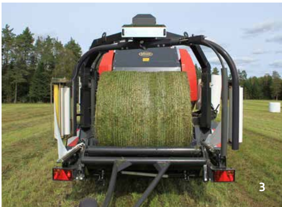
As soon as the bale is transferred away from the baler, the tailgate automatically closes, and the baling of the next bale can start.
