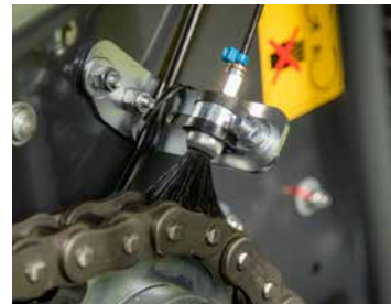
Automatic chain lubrication is standard on FixBale 500.
