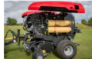
Easy access storage for net and twine for long working days.
