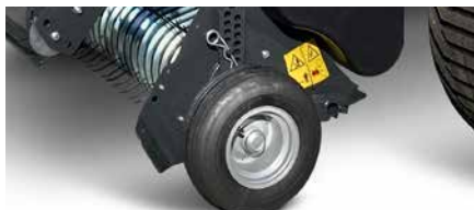
Large diameter easily adjustable guide wheels.
