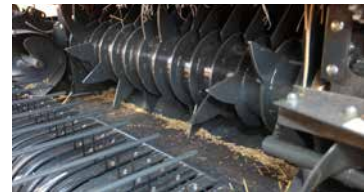
PowerFeed intake system.
