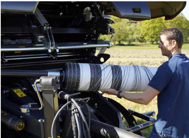
Very low loading height and easy threading of the system make for minimum downtime and maximum time baling.
