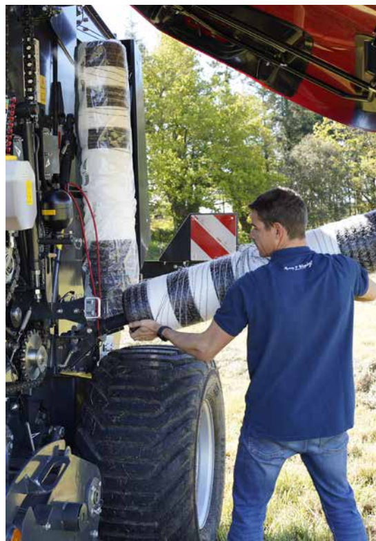
The smart net roll storage allows a comfortable horizontal loading.
