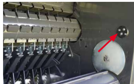
Moisture sensor located inside the bale chamber.
