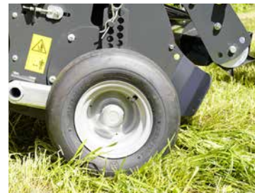
Generous flotation tyres with simple height adjustment.
