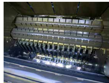
Profiled rollers provide instant bale formation and are equipped with self cleaning scrapers designed for working in all crop conditions.
