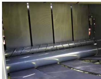
Spiral profile scrapper roller for efficient cleaning effect in all condition.
