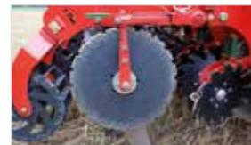
The **side blades** Ø460mm retain loose soil in the strip and define width and form of the strip via the angle and depth adjustment of the disc.
