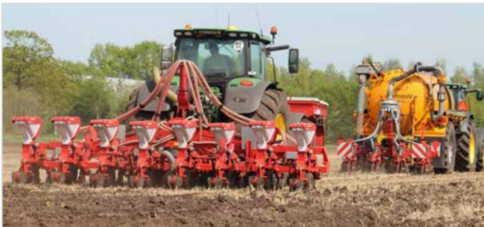
By using GEOCONTROL® there are no overlaps. Costs for fertiliser, seeds and chemicals are saved as well. GPS control of the tractor is advised for the Strip-Till. The implementation of the RTK signal (+/- 2cm) guarantees high precision. The working width of the Strip-Till implement should correspond to the working width of the precision seed drill or have its double width at maximum.
