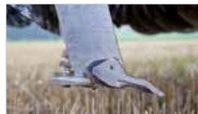
Special **tines with shares** break-up the soil down to a depth from 10cm to 30cm. Three different type of tines and a hydraulic overload protects the loosening leg. For a longer lifetime a carbide version is available.
