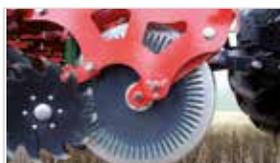
The **front-cutting discs** open the soil and cut long residues which can be easily removed by the following trash wheels.
