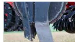
Two options of **fertiliser lances** are available. A smaller one used for granule mineral fertiliser and a larger one (60mm) for the injection of slurry. Depth-setting (0-20cm) independent of working depth. The fertiliser is placed during strip cultivation.
