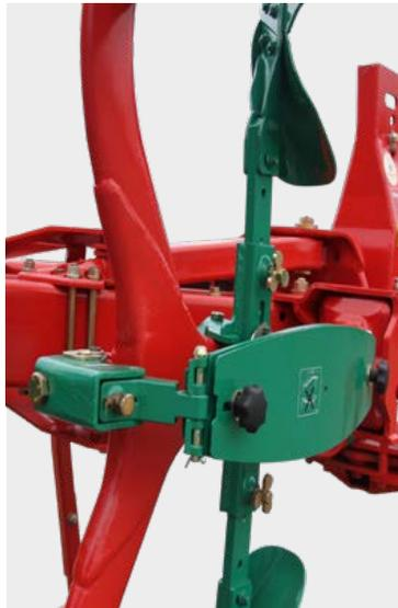
The new generation of Kverneland ploughs feature legs with a new design, called "aero-profile". Not only higher than the standard Kverneland legs, these new legs improve the soil flow. Heavy residues are pushed out, hence limiting possible blockages even with 85 cm interbody clearance.
