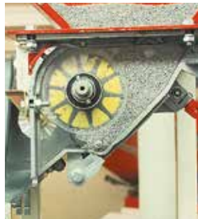
Setting for fine seeds, with rotary brush
