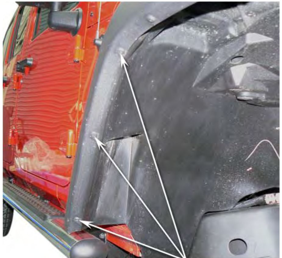
Remove Plastic Pop Rivets
