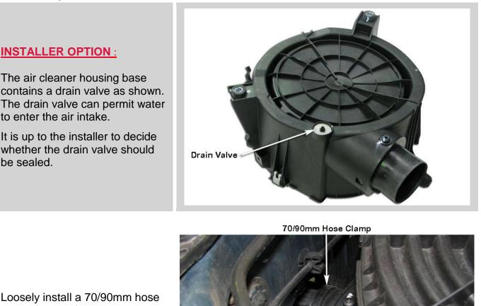
Loosely install a 70/90mm hose clamp (Item 11) over the air cleaner inlet adaptor, install the air cleaner base into the vehicle and fasten with standard mounting bolts.
