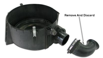
Remove and discardAir intake duct
