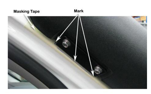
Position the upper mounting bracket onto the A-Pillar and align the bracket with the marked bracket outline. Mark the three mounting hole positions with a felt tip pen.
