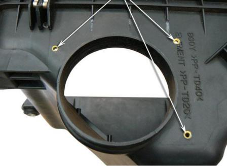
**13** Apply a liberal amount of adhesive sealant to the air cleaner adaptor flange (Item 12) and around the external surface of the air cleaner inlet snout.
