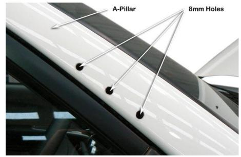
**10** Secure the upper mounting bracket (Item 3) to the A-Pillar using 3 x self tapping screws (Item 5)
