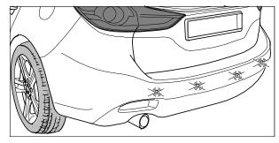
On the facelift GL models the PDC or SCBS-R system is not active while the parking brake is engaged.
