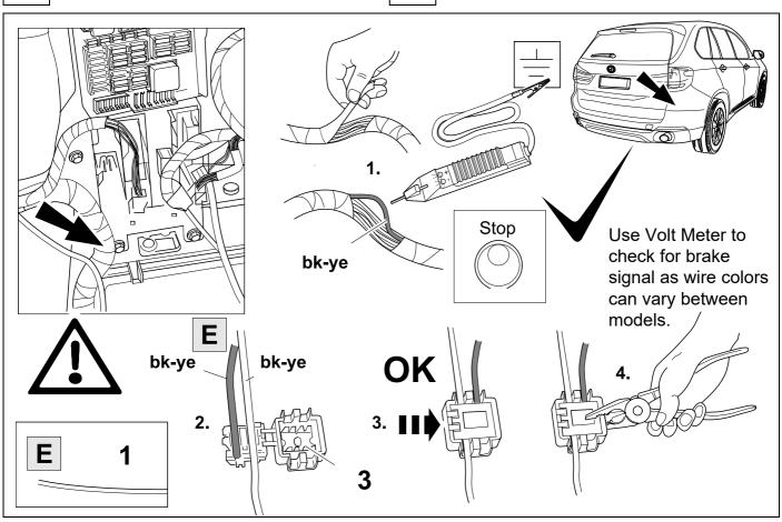
Use Volt Meter to check for brake signal 15 as wire colors can vary between models.
