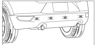
The PDC or SCBS-R system is not active while the parking brake is engaged.
