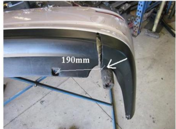
drivers side mark out, then draw staight line between marks, then mark 25mm towards center
