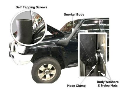
Align the two hoses (items 10 &12) for best fitment, ensure that the snorkel outlet hose (item 10) is installed hard up against the shoulder of the snorkel body outlet snout, tighten the 90/110mm hose clamp (item 14).
