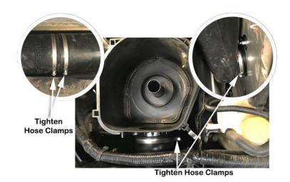
Install the black hose clamp (item 15) loosely over the base of the air ram assembly (item 2).
