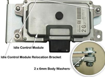
Assemble the idle control module to the relocation bracket (item 24) with three 6.0mm x 20mm hex bolts, (item 27) and three 6.0mm body washers (item 29), install the bolts with washers installed through the bracket, install two 6.0mm body washers to each of the bolts for spacers, and install the idle control module. Install a 6.0mm body washer and a 6.0mm nyloc nut (item 30) to each of the bolts.
