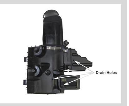
32 Install the air cleaner base and hose assembly into the vehicle. Hint: squash the end of the hose whilst installing through the hole in the inner guard.
