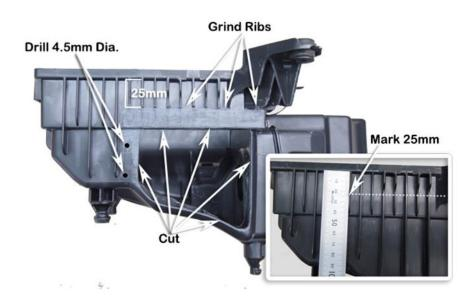
Using a body saw or die grinder remove the ribs as shown.
