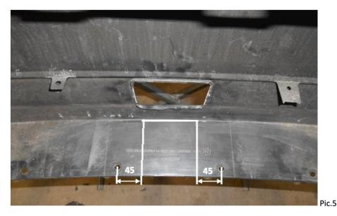
5.1 Measure from the holes towards the centre of the bumper bar 45 mm as shown on Pic.5
