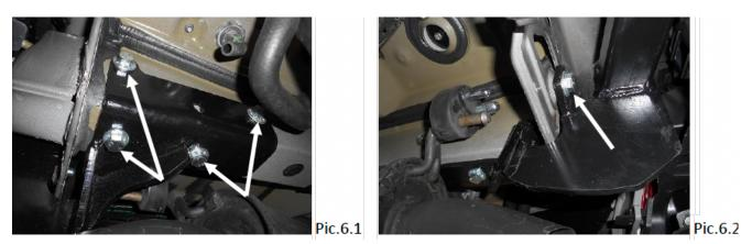
5.1 Slide the towbar between the chassis rails and insert fasteners as shown on
